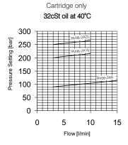
The Performance Chart illustrates flow handling capacity at max. setting for each spring range option. Pressure rise will vary with spring (range) and with setting within range due to flow forces.
